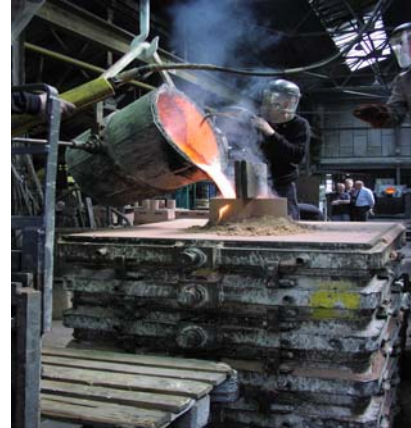
Casting into a Patternless® mould
